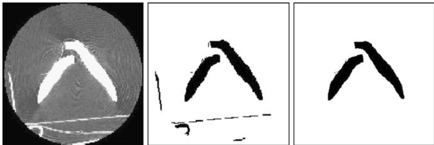
Fig. 4.4 (a) A typical 2D CT slice from a phantom CT sequence. (b) The CT slice after simple thresholding. (c) The CT slice after connected component labeling and size filtering. In (b) and (c), the grayscale value 0 (i.e., color black ) is used to represent the mandibular bone fragments and artifacts
